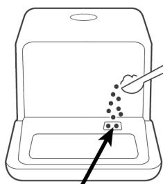
The appliance requires less detergent than commercially appliances. Normally one tablespoon of detergent is enough for a normally dirty rinse load.
