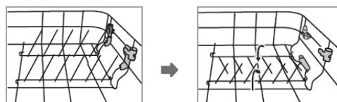
To create a better arrangement for bulky dishes, the rack shelves can be folded. Lift the racks slightly and fold them down.
