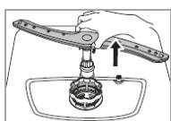
Lime and impurities from the rinsing water can block nozzles and bearings of the spray arm. Check the outlet nozzles of the spray arm regularly for blockages.
